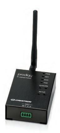
The Prodigy P-MNETGW is a 2-way gateway transceiver that provides communications for the complete line of Prodigy wireless devices with the PMC2 Prodigy Media Controller.
