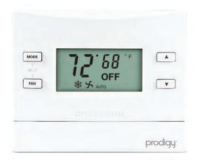
The P-TSTATRF is a wireless thermostat that makes it easy to add networked climate control to any home. Mesh network technology of 802.15.4 affords reliable communications and temperature control without the need for additional wiring. Whether installed in retrofit or new construction, the P-TSTATRF provides a climate control solution and the benefits of intelligent control for any budget.
